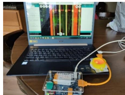
Figure 2. ERG setup. Light stimulator flashing red light (right), Spikerbox (bottom), and ERG data acquisition (screen).
